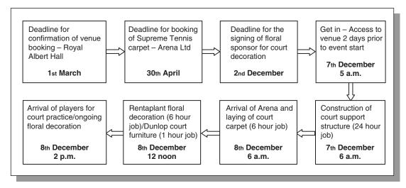
**Figure 8.1** A critical path – Nabisco Masters Doubles. A network depicting one sets of tasks – the construction of the tennis court for the event at the Royal Albert Hall. The critical path is represented by the arrow and shows that the failure of one task impacts on those that follow
